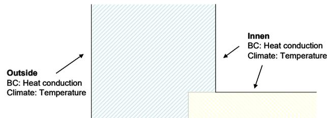
At symmetry lines and at borders of the calculation domain (where 1D conditions are expected) boundary conditions are not needed. A boundary without assigned boundary conditions is perfectly tight and adiabatic. In this example only heat conduction boundary conditions with the corresponding temperatures are needed.
