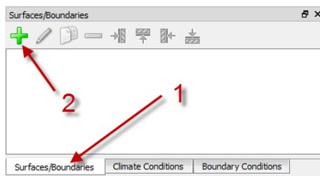
As with all definitions in DELPHIN, give the new interface a unique description name, for example “Inside”. Then, select the type of surface/boundary. In this tutorial, we have created boundary conditions manually, so we use **Detailed/scientific interface**. Afterwards check the boundary conditions that shall be associated with this interface/surface. For the inside surface, check “Indoor heat conduction” and “Indoor vapor diffusion”.
