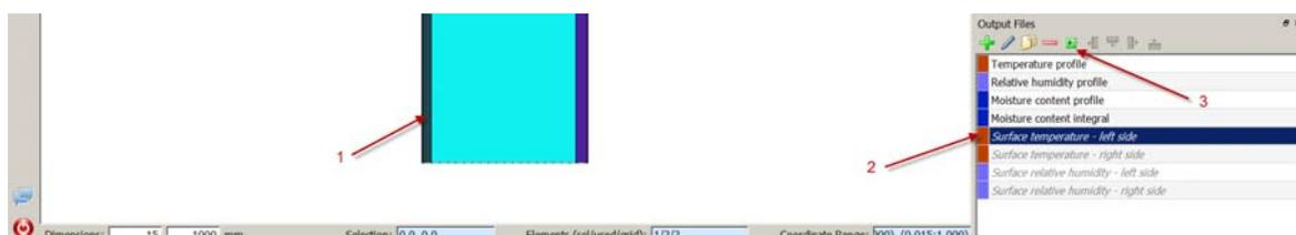
After clicking on the assignment button a dialog will occur. Here one can decide if the output should be related to a volume element or to a position. For a surface output a position related assignment should be used. The coordinate
