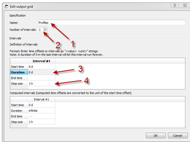
For each interval, you need to select the duration of the interval (3) and the output step size (4). Alternatively, you can specify start or end times of intervals, whereas time means relative time since start of the simulation.
