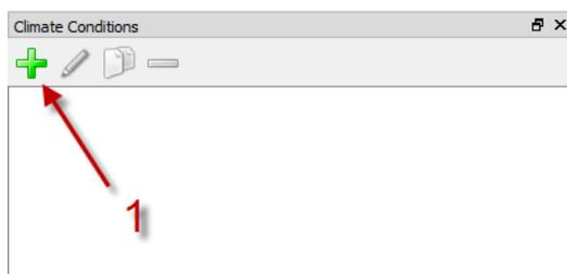
Doing this for Climate Conditions open the dialog for climate data. There you can specify the climate data, basically a single climatic data component: identification name (1), **Temperature** as type of quantity (2), variability in (3) where we use **Constant** and finally the value in (4).
