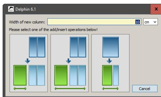
In the input line above you can specify the thickness of the new layer. Below it there are three graphic buttons that show how to use this thickness:
