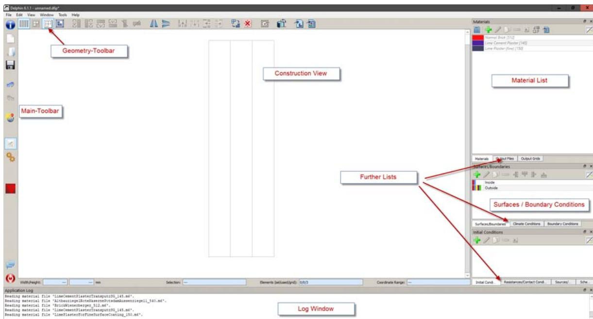
The layout of the windows can be adjusted at will. The various definition lists can be shown/hidden via the Window-menu on the upper left. Also, they can be dragged around and put together in tabs. For this and the following tutorials, we will use the standard layout.
