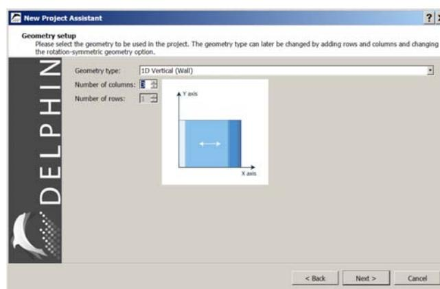
Here one can select the basic geometry type and the main construction grid. We want to calculate a one-dimensional wall structure therefore 1D Vertical (Wall) should be selected. The type of construction can be changed at any point in time later. The existing historic construction has 3 layer (columns). The thicknesses of these layers can be edited later. In the next dialog the boundary conditions can be set.
