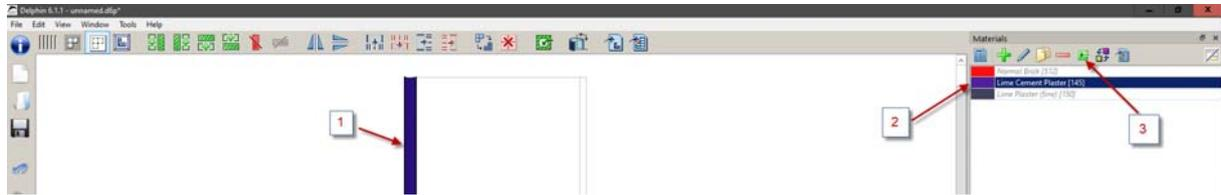
To do this, you need to select a layer (or several layers) with the mouse (1). Then select the desired material in the material list (2) and finally press the green assignment button (3). The order of the actions can be reversed as well.
