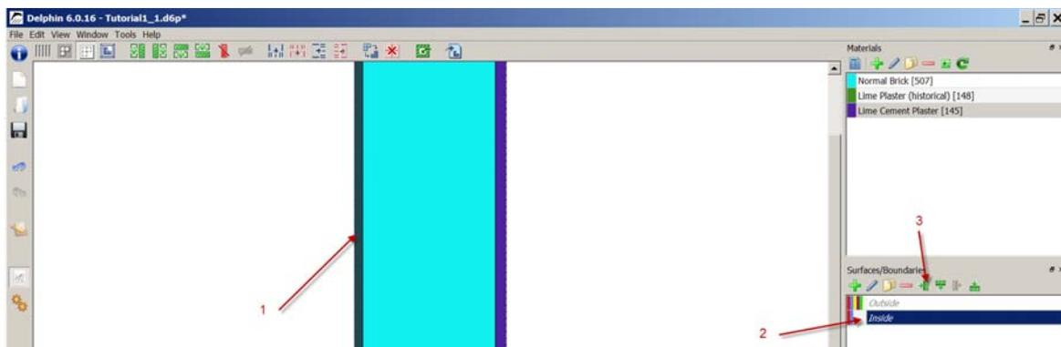
The inside climate will be located to the left. Select a column (1), select the interface to assign (2) and last click on the button for assignment to a left side (3). Proceed with the right side for the outside interface. One can check if the interface is assigned correctly by clicking on an interface in the ‘Surface/Boundaries’ list. The interface will be marked in the construction view with a dashed line (see picture below).
