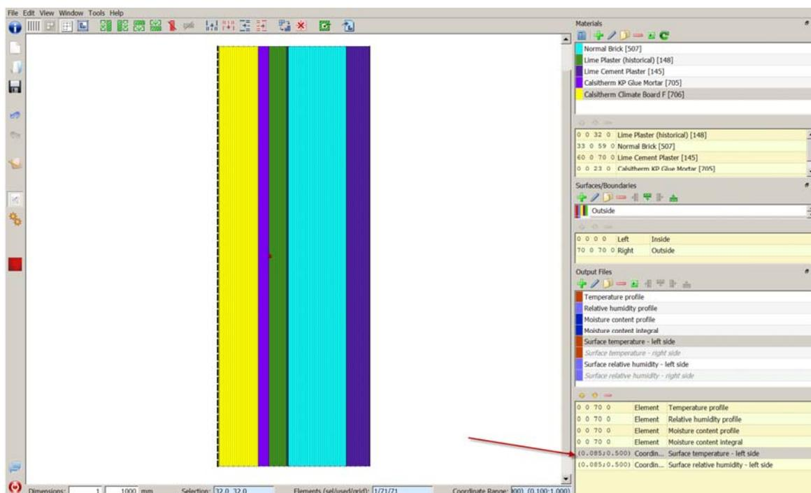
The red arrow marks the position of the assignment parameter for the (former) surface outputs. As you can see the x-coordinate now is set 0.085 m. This has to be changed to 0.0 m: double-clicking on the assignment allows you to edit values.
