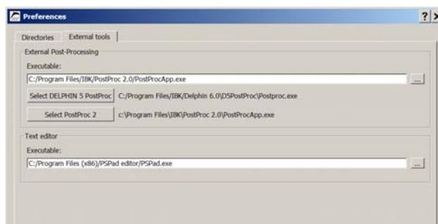
Click on the corresponding button of the post-processor version to select it. After opening the PostProc 2, the data of the current project should normally already be loaded. If not, these data must be loaded from the project directory.
