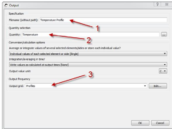
Next you have to select the physical quantity for the output (2). In the quantity selection list that is opened with the associated button, you see all the quantities that can be calculated with DELPHIN.
