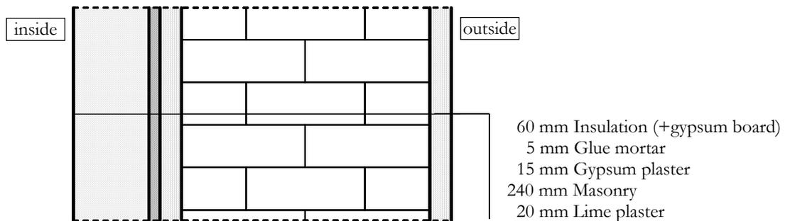
First, the previous construction (without inside insulation system) shall be evaluated with respect to its hygric and thermal performance. Afterwards a variation study is done to find a suitable inside insulation system.
