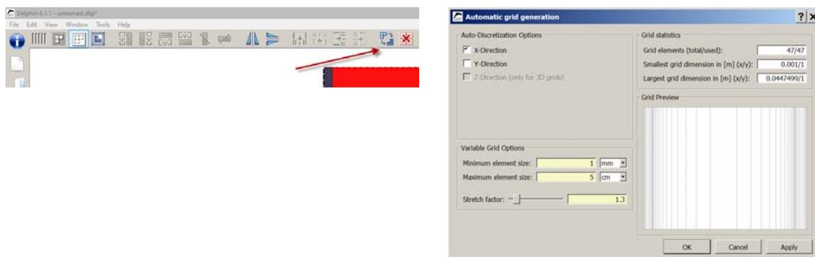
In the Automatic Discretization dialog we will only discretize the construction in X-direction - as we have to deal with a wall with horizontal transport direction only. We use variable discretization that generates smaller elements near the boundary of the construction and at material interfaces. Inside of the construction the element widths are gradually enlarged.
