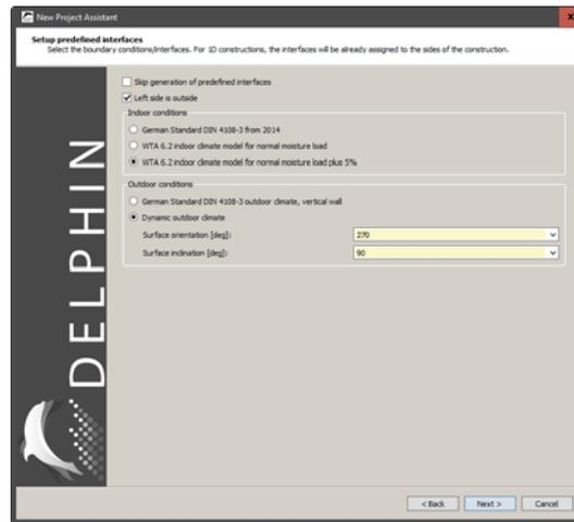
Checking the topmost selection skips this process. The boundary conditions must then be defined manually. In the second selection box you can define where the outside should be. If this box is checked, outside is on the left side, otherwise it is on the right. In this tutorial the left should be inside, so the hook must be removed. Afterwards the indoor climate and the outdoor climate are set. Here the following is selected:
