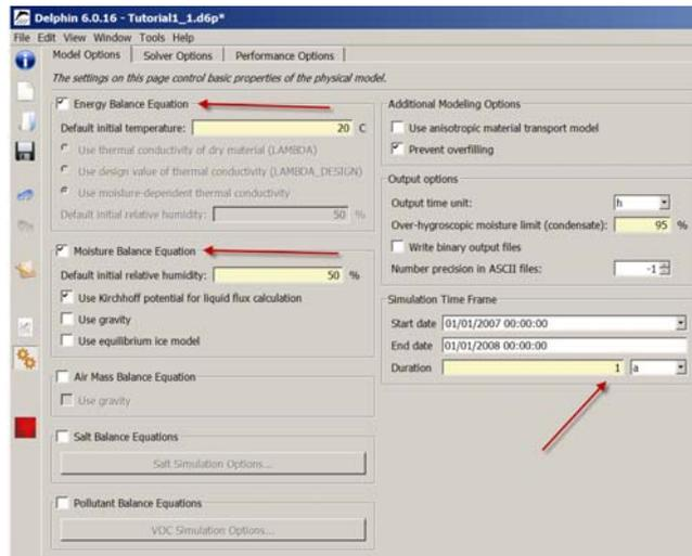
Other important settings in this dialog are the duration and the starting time of simulations. Here, we use only one year as duration of the simulation. The starting time is not important for a design simulation. However, the initial conditions need to be specified. They can be set globally in the “Defaults” section of the balance equation
