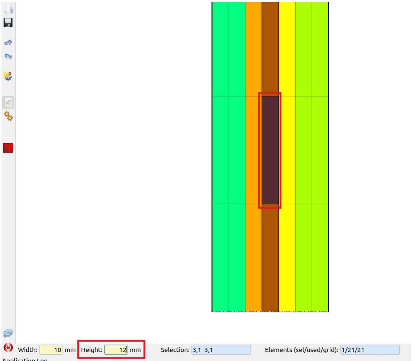
Figure 8. Adjusting the height of a row
