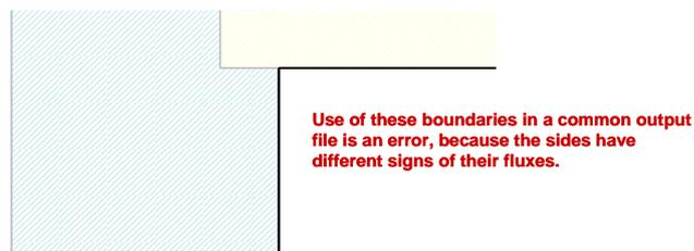
If the construction were defined as above, the assignment would be wrong. A heat flux from the inside to the outside would yield a positive flux for the top interface (flux in positive y-direction), yet the flux through the vertical interface would yield a negative flux (against the x-direction). When you add these up in an integral heat flux output the flux would cancel each other, even though both flux indicate a positive energy flux from the inside to the outside.
