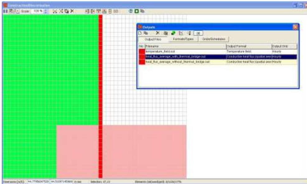
For comparison you can create another output just for the inner boundary element of the first row. Here we are far away from the thermal bridge and should have (approximately) one dimensional conditions. A heat flux obtained here corresponds to the heat flux of the wall without the thermal bridge. We can use this as reference value for the rest of the wall.
