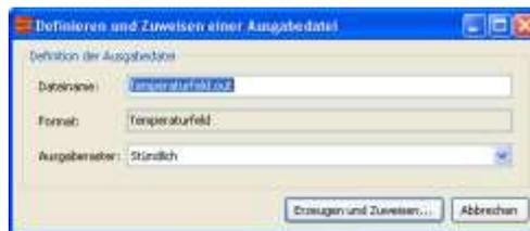
Sometimes you may just want to obtain an output of a part of the construction, for example, the total moisture mass in a certain material. In our case, we could just want to obtain the temperature field of the aerated concrete (even though this doesn't really make much sense). However, we have to assign an output now to an element range that is not rectangular. So we have to make two assignments. For such cases, the following procedure is recommended:
