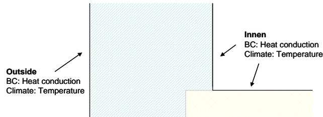
At symmetry lines and at borders of the calculation domain (where 1D conditions are expected) you do not need to assign boundary conditions. A boundary without assigned conditions is perfectly tight and adiabatic. In our example we just need heat conduction boundary conditions with the corresponding temperatures.
