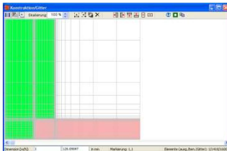
The first top tool buttons
