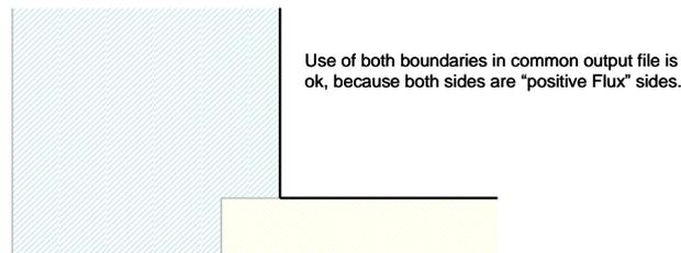
Both boundaries have the same sign definition which allows us to combine the two outputs into a single file for the integral heat flux density.
