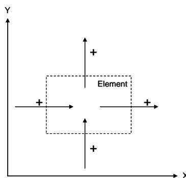
This sign definition is used independently whether a side is between two elements or a boundary side. Flux densities in direction of the coordinate axes are always positive. That has the advantage that one can define cut planes through
