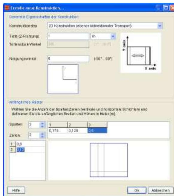
When entering the basic grid geometry you should note that the **grid widths and heights are in m**.
