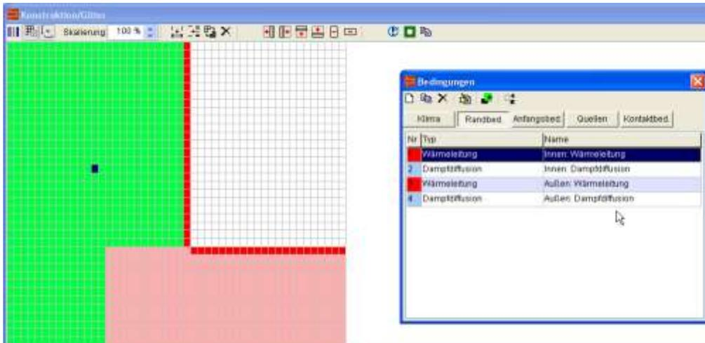
In the assignment list window you can also check all assignments individually. There should be 3 boundary condition assignments in total: one for the heat conduction at the outside, and two for the heat conduction at the inside, just as it is shown in the screenshot above.
