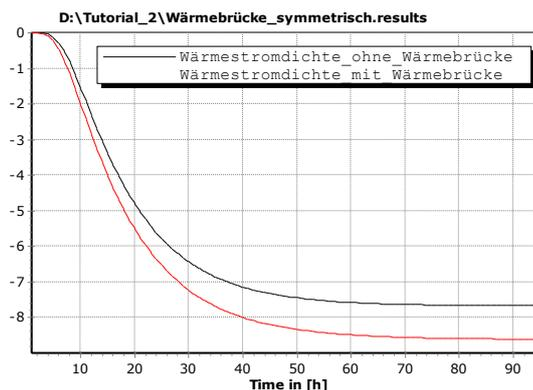
Also, we see that the thermal bridge does increase the heat flux through this part of the wall by about 12 % compared to a plain wall (red curve is the output with thermal bridge, black is the reference).
