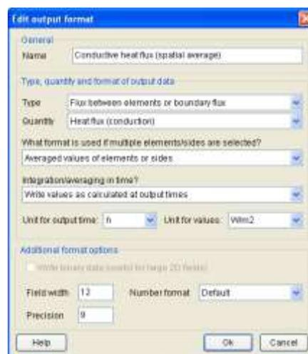
When defining the output it is important to set the output type to a "Flux type" and select the weighted average as calculation method.
